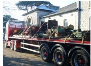
23 January the engine was again taken apart and loaded on to lorries for the journey to its new home. To give you an idea of scale, the load on the lorry with the frame 10 tons, while other. with the flywheel at the front, and cylinders in the middle weighed in at 26 tons. John says that he is now hopeful that the engine will have a certain future, despite this being away from where it spent its working life. All that now remains is for SPAM to organise a trip to see it in its new home!
