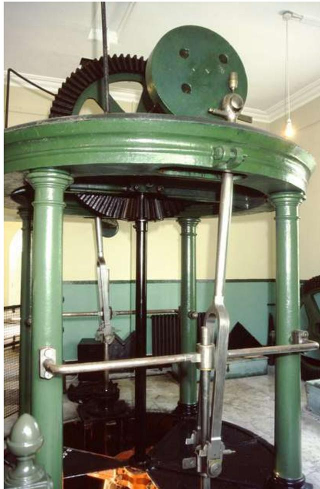
The 1857 turbine-driven water pump, manufactured by D Crook of Glasgow
